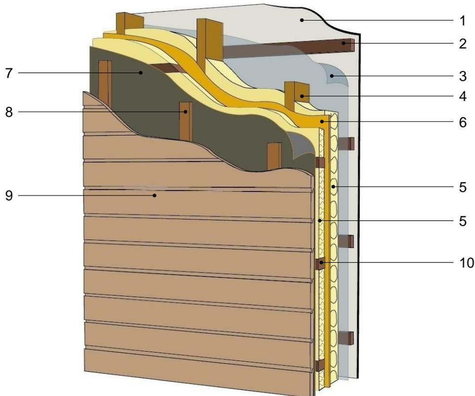
**DEFINITION DES COMPOSANTS DE LA PAROI CONFORMES AU CGM DU NF DTU 31.2 ET NOTAMMENT AUX CARACTERISTIQUES CI-DESSOUS**
