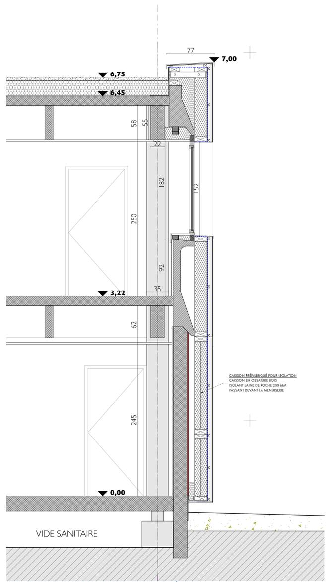
PROJET \_ COUPE DE PRINCIPE / ISOLATION PAROI PLEINE EN RDC POUR CONTINUTE DE FACADE
